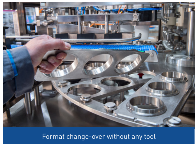
Format change-over: several cup diameters are possible in a Serac cup filler
